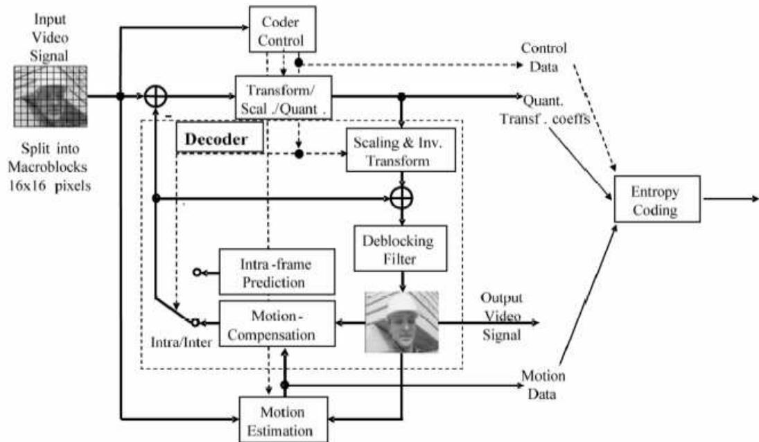
Figure1. Basic coding structure for H.264/AVC for a macroblock.
